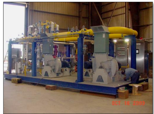
ONE SINGLE SKID FOR AFCU, AMMONIA VAPORISATION & DILUTION
